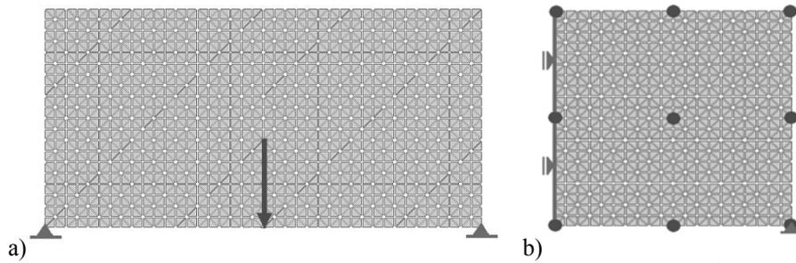
Figure 6: The plate (example 1); a) the geometry; b) the distribution of the control points of the interpolation surface
