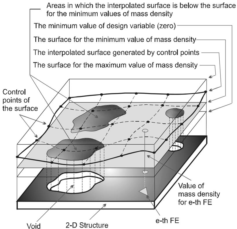
Figure 2: The illustration of the idea of immune optimization for a 2-D structure
