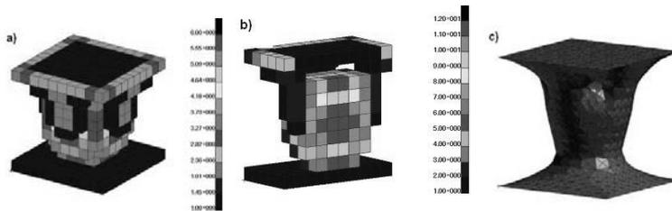
Figure 9: Distribution of mass density for the first case (compression) a), b) structure after 50 iteration (the best solution) c) structure after smooth
