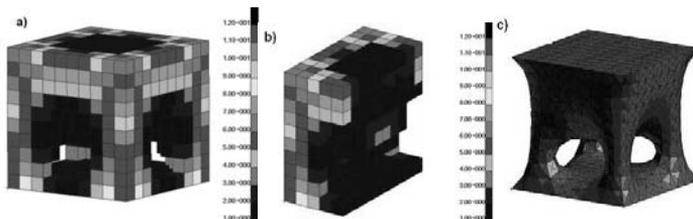
Figure 10: Distribution of mass density for the second case (tension) a), b) structure after 50 iteration (the best solution) c) structure after smooth
