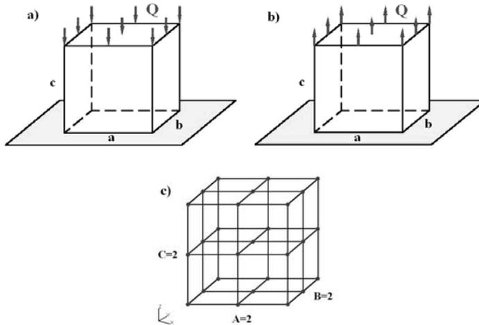
Figure 8: Two cases of loading with the hyper surface a) first case (compression), b) second case (tension), c) the distribution of the control points of the interpolation hyper surface
