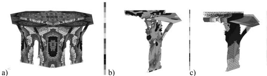
Figure 12: The results of the immune optimization of the shell-solid structure: a) the solution of the optimization task; (the map of mass densities); c) the map of stresses; d) the map of the displacement
