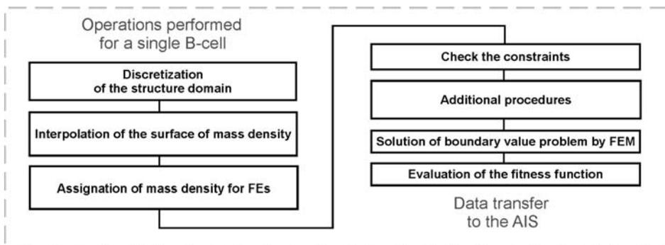
Figure 3: Operation scheme performed for a single B-cell
