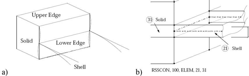
Figure 1: Shell-to-solid transition: a) clamped connection of a shell to a solid, b) best modeling practice for RSSCON
