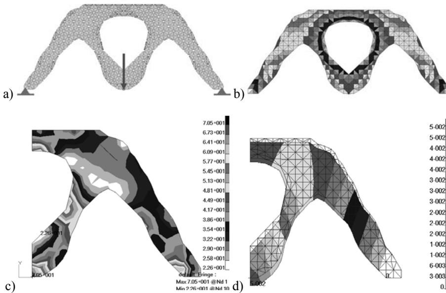
Figure 7: The results of the immune optimization of the plate: a) the solution of the optimization task; b) the map of mass densities; c) the map of stresses; d) the map of the displacement
