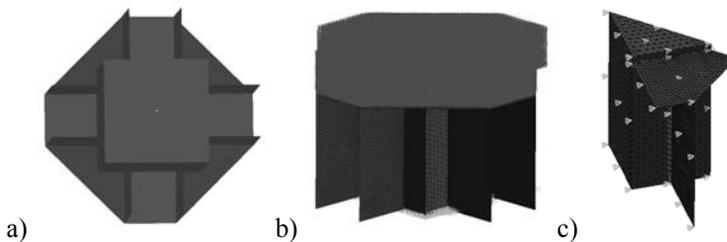
Figure 11: The shell-solid structure (example 3); a) the geometry; b) the boundary condition; c) the distribution of the control points of the interpolation hyper surface
